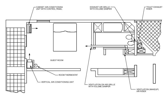
Fig. 2 Alternative Location for Hotel Guest Room Air-Conditioning Unit on Room Perimeter and Chase-Enclosed
