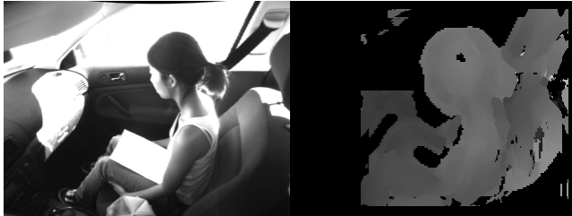
Fig. 4. Example of reflectance and corresponding disparity images for a subject in the LISA-P test bed
