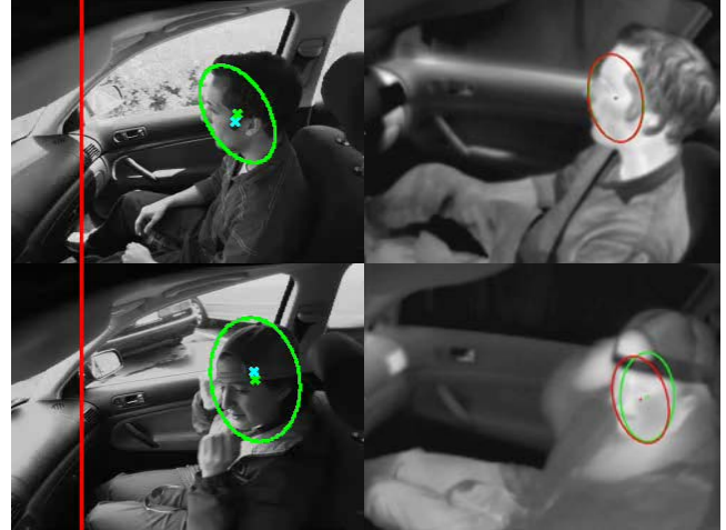
Fig. 8. Example images of successful head detection for both the stereo and LWIR based algorithms. The top pair show successful detection for sitting normally, and the bottom pair shows successful detection when putting on a hat.
