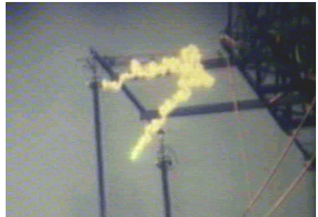
Figure 4: Secondary arc in middle velocity (3-4 m/s) wind along a 400 kV non-ceramic insulator
