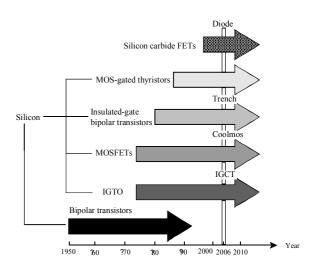
Fig. 3. Development of power semiconductor devices in the past and in the future [34]
