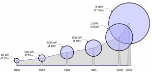
Fig. 16. Development of wind turbines during the last 25 years.
