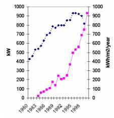
Fig. 14. Average size of wind turbines and produced energy pr.
