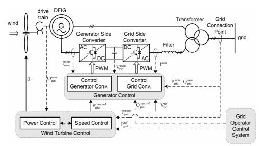
Fig. 10. Control of wind turbine with doubly-fed induction generator system [35].
