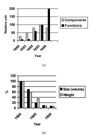
Fig. 2. Development of a 4 kW standard industrially adjustable speed drive during the last 25 years [5].
