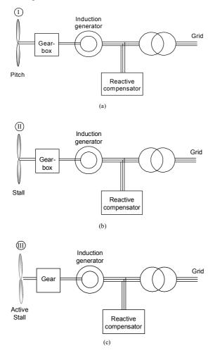
Fig. 6. Wind turbine systems without power converter but with
