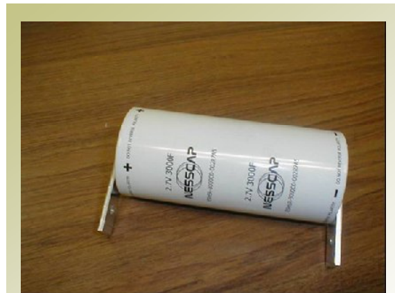
Figure 2 The NessCap 3000F capacitor
