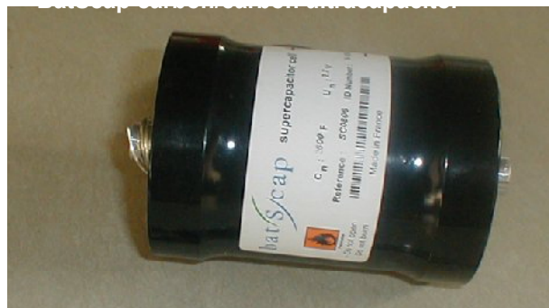
Figure 3 The Batscap 2700F capacitor
