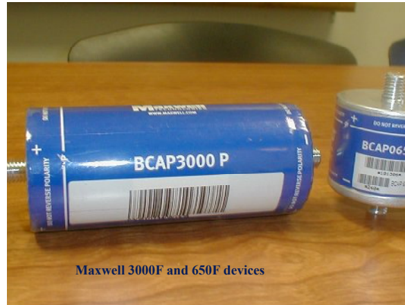
Figure 1 Maxwell 3000F and 650F capacitors
