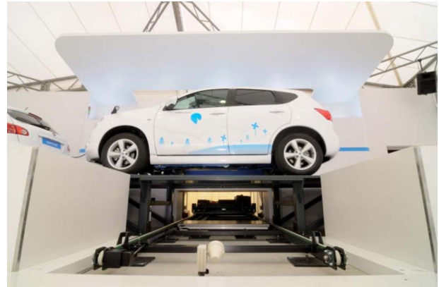
Fig. 5. Better place battery swap station. Photo courtesy of Better Place.
