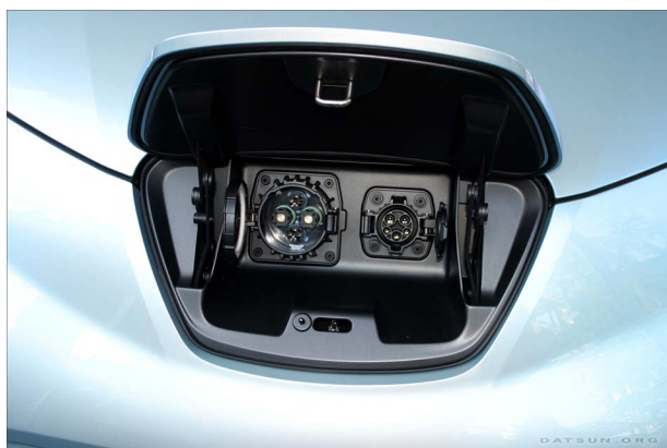
Fig. 8. Nissan leaf fast charging JARI CHAdeMO plug (left) and SAE J1772 Level 1/2 plug right. Used with permission from Datsun.org.
