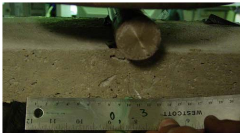
Fig. 22. After the loading: the crack almost disappears.
