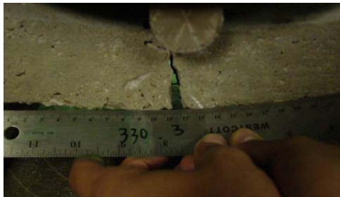
Fig. 21. During the loading: the crack can be obviously seen.
