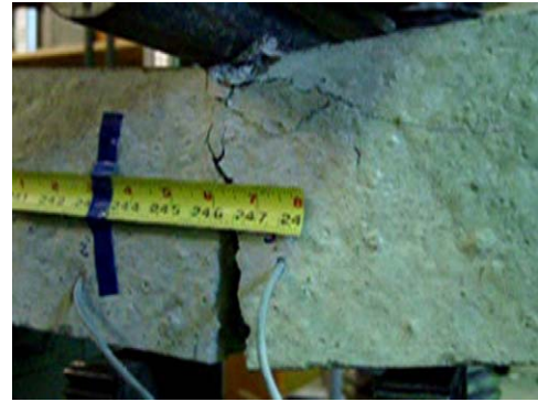
Fig. 16. A large crack during a loading test.
