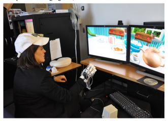
Figure 1. System and interaction with the VR environment. User wears a custom pneumatic glove, which assists finger extension. Magnetic trackers provide information regarding head orientation and hand location; the virtual scene is updated accordingly.
