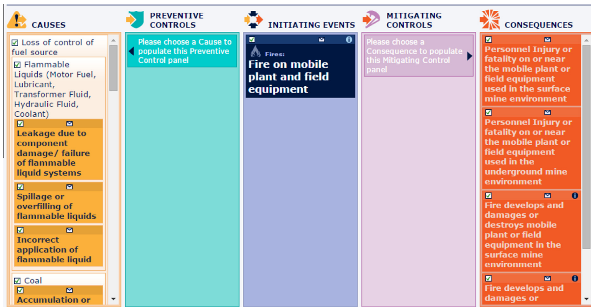
Fig. 5. Example of the RISKGATE system's use of bow-tie analysis for graphic representation.
